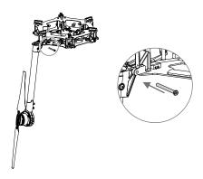
d. Gently lift the frame arm and twist the red knob to lock the arm in place.
