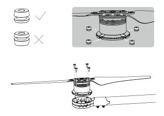
$\underline{ }$  Ensure that all dampers are in good condition before every flight. If they are not, they may adversely affect flight performance and should be replaced immediately.
