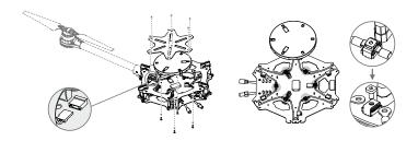
d. Unscrew the M4×35 screw and remove the original frame arm.
