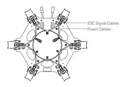
i. Replace the round cover and tighten the four screws (M3×8 self-tapping), then replace the upper plate of the center frame and tighten the six screws (M2.5×8 cheese head).
