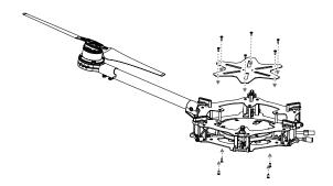
j. Double check all frame arms. Arms M1 and M2 correspond with the nose direction of the aircraft. Arms M4 and M5 correspond with the tail. When viewed from above, the motors on arms M1, M3 and M5 should rotate counter clockwise and the motors those on arms M2, M4 and M6 should rotate clockwise.
