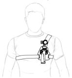
To remove the Osmo, loosen the knob and toggle the lock button to its unlock position, then remove the Osmo while pressing down the lock button.
