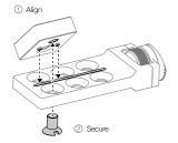
Make sure the Mounting Adapter is secure before attaching your accessory.
