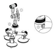
Place the Vehicle Mount on a flat surface such as the roof of your car. Ensure the suction cups make good contact with the surface and then push down the suction cup levers.
